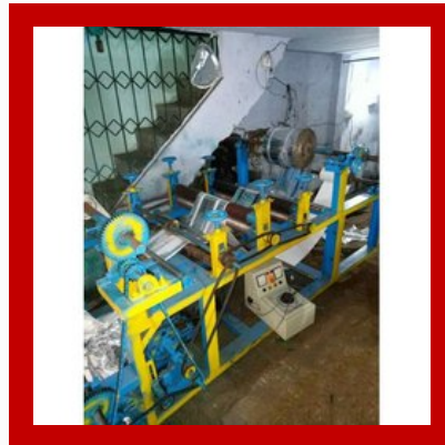
Paper Plate Lamination Machine
