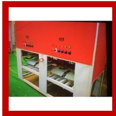
Four Die Paper Plate Making Machine
