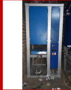
Fully Automatic Single Die Paper Dona Making Machine
